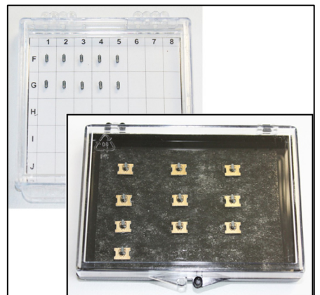
10 self-sensing cantilevers (STD on PCB, optional as Si-chips), Si-chip h=0.3 mm
